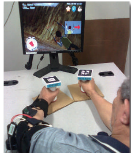
Figure 1: A stroke patient using the Neurorehabilitation Training Toolkit (NTT), a VR upper limb motor rehabilitation system for training bimanual coordination.
