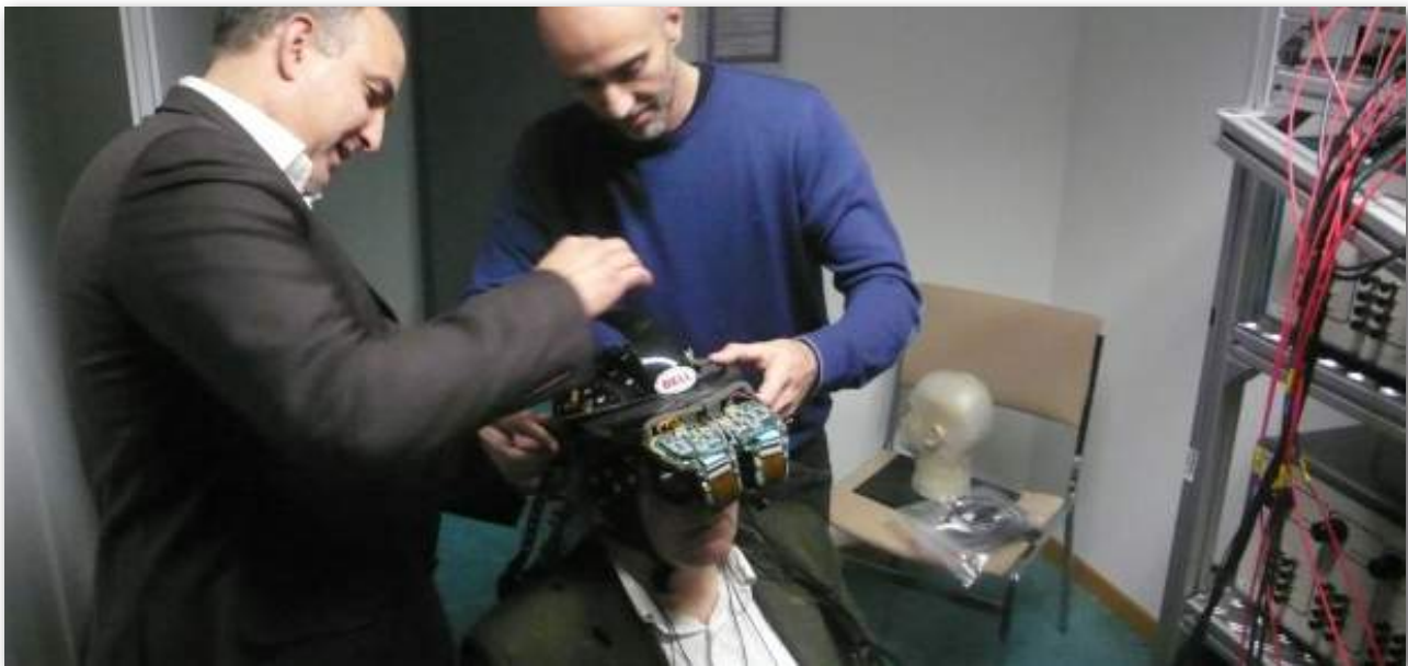
Figure 1: Setup of fNIRS (Functional Near Infrared Spectroscopy) and VR (Virtual Reality)
