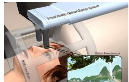
Figure 1: VR compatible MRI scanner with subject looking into VR goggles
